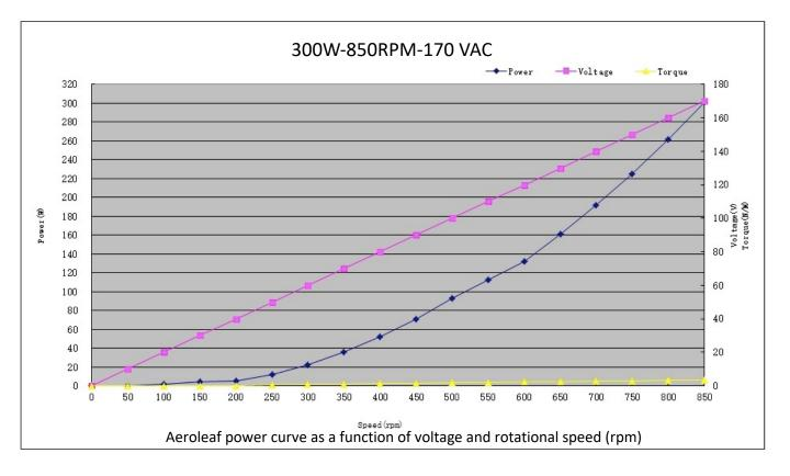
Every 10 milliseconds, the microprocessor calculates the voltage/current relationship to instruct the Aeroleaf to reach the best rotation speed compared to the ideal power extraction curve.
